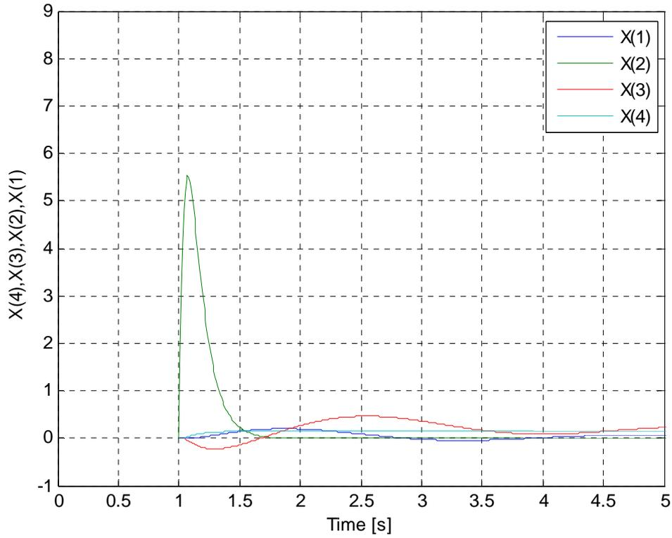
Fig. 14 : The response of aircraft states for the case of LQR-ABC
