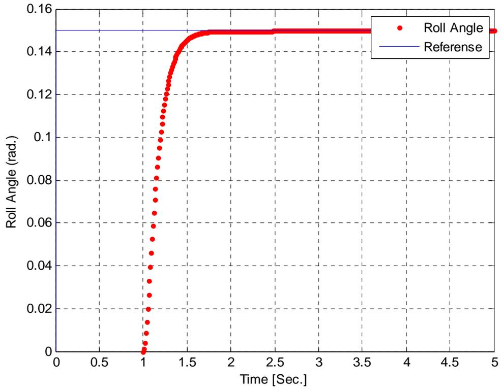
Fig. 6 : Step response of the roll angle for the case of LQR-GA
