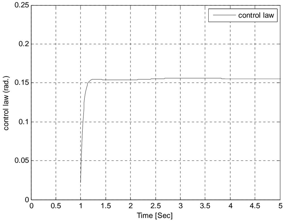
Fig. 10 : The response of the control signal for the case of LQR-PSO
