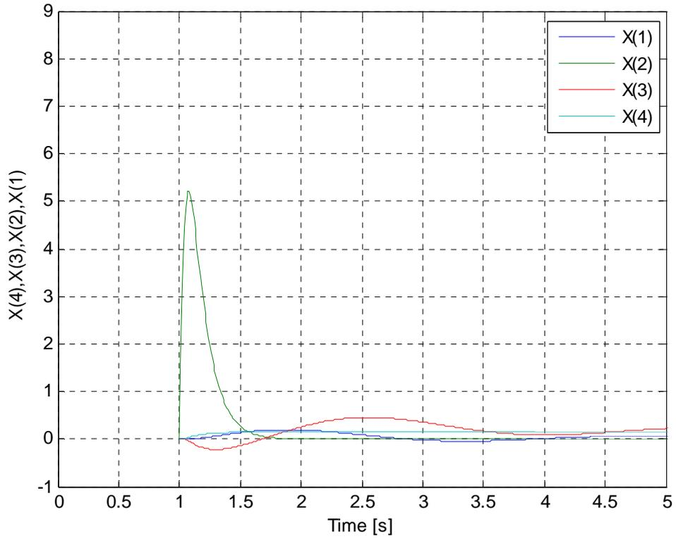
Fig. 8 : The response of aircraft states for the case of LQR-GA.
