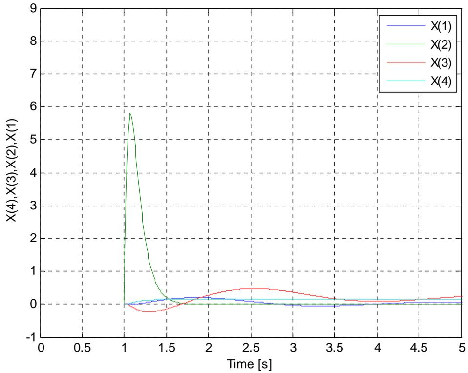
Fig. 11 : The response of aircraft states for the case of LQR-PSO
