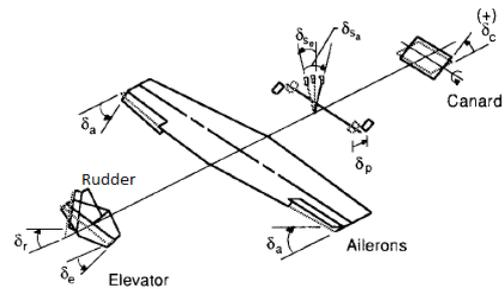
Fig. 1: Control surfaces of an aircraft system [1]
