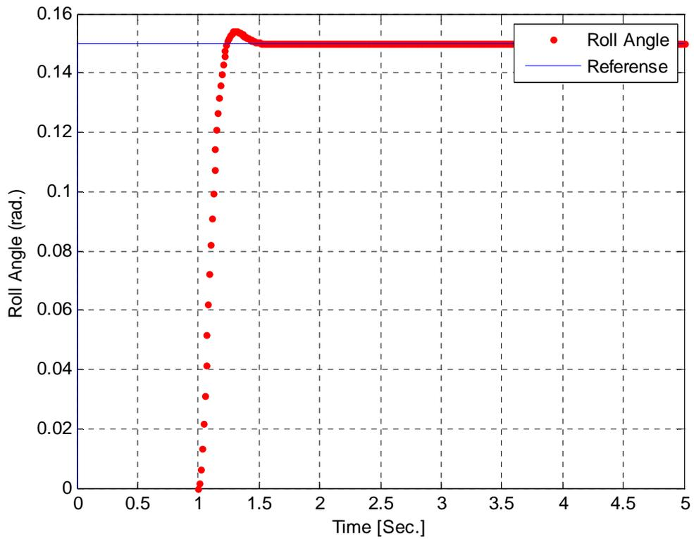
Fig. 3 : Step response of the roll angle for the case of LQR of [5]
