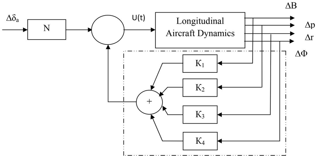
Fig. 2: Roll Control system with full-State Feedback Controller of Reference Input
