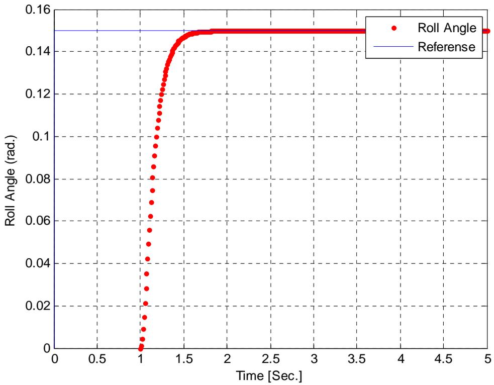
Fig. 9 : Step response of the roll angle for the case of LQR-PSO.
