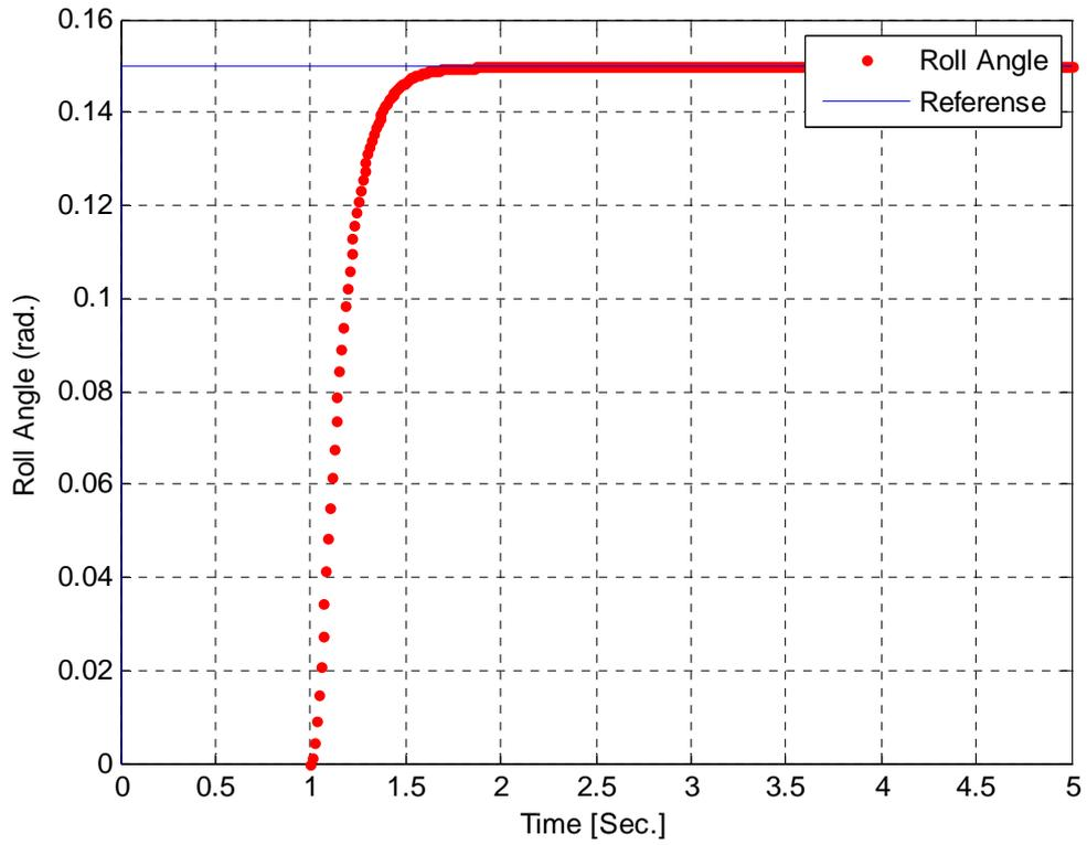
Fig. 12 : Step response of the roll angle for the case of LQR-ABC
