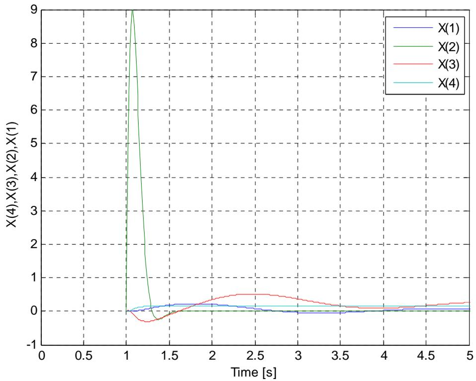
Fig. 5 : The response of aircraft states for the case of LQR of [5]
